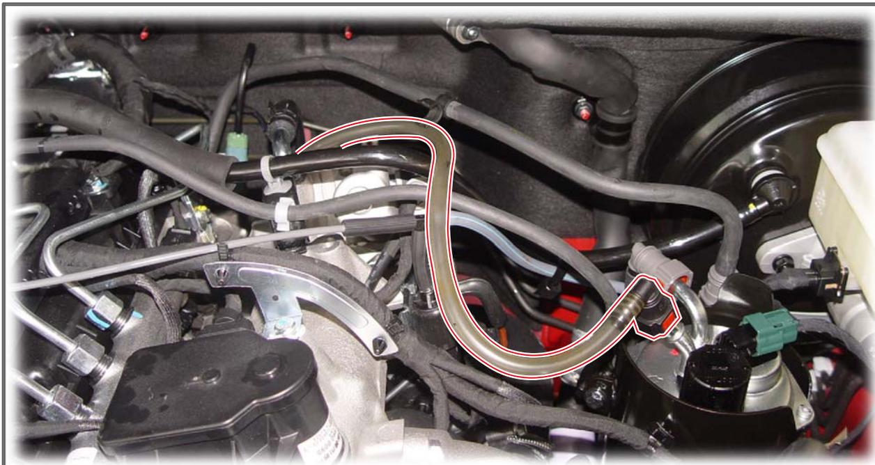
4. Start the engine and check visually for clogged low pressure fuel system, excessive air or air entry. If the fuel flow is not sufficient or air is in the fuel, repair the leak area.
