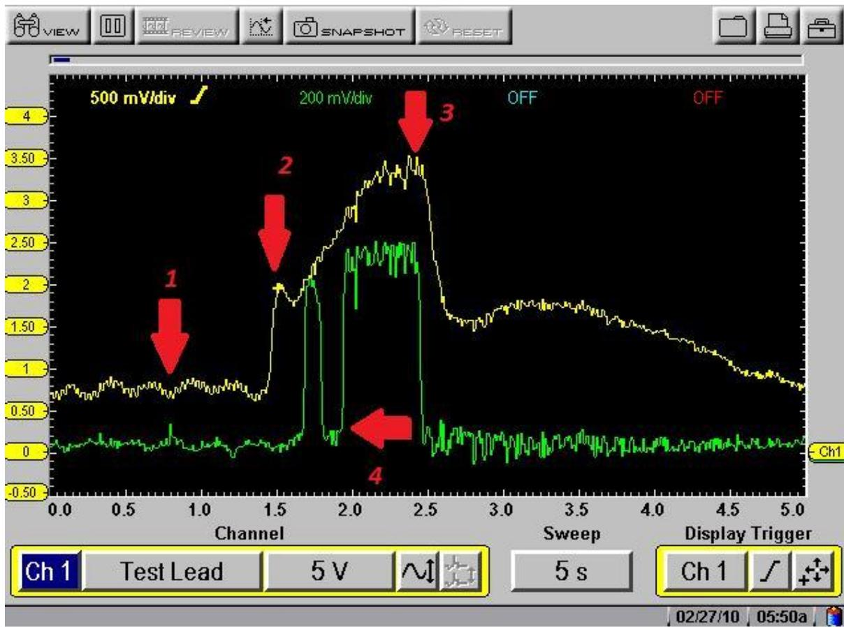
The image above shows a faulty mass airflow meter fitted to a 2004 Opel/Vauxhall Vectra Z16XE. The yellow trace is the mass airflow meter (MAF) signal and the green trace is the pre-catalyst exhaust gas oxygen sensor.
